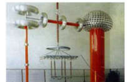
Power frequency withstand voltage inspection
